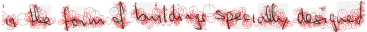
Figure 1 Cropped example of a text line with the detected IP and their dominant orientations denoted as circles, where the size indicates the scale, and the line originating from the center the dominant orientation. Several orientations indicate multiple IP with different dominant orientations at the same location.
