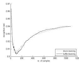
Figure 3. Comparison of recognition rate between block and buffer-based learning.
