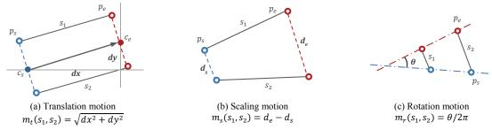
**Figure 2.** Three types of motion between sub-strokes,  $p_s$  and  $p_e$  represent the start points pair and end points pair, respectively. Since all the gestures are normalized inside a unit square bounding box, these three values have the same range in [0,1].
