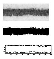
Figure 2. An image used in the experiment and pre-processing. The top column: raw image, the middle column : binary image, and the bottom column : contour image
