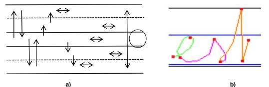
**Figure 1** The "zone" features. a) The features: their labels depend on both the writing direction (represented by the arrow) and the zones of the stroke extremes. The arrows are not representative of the actual shape of the strokes. b) the partitioning into subsequences: begin (green), middle (magenta) and end (yellow)
