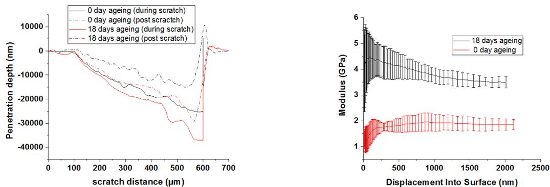
**Figure 2: nanomechanical test recorded on 0 day or 18 day ageing PP under weathering accelerated chamber a) Evolution of the Young's modulus as the indentation depth b) the scratch profiles (solid lines) and post scratch profil (dashed line).**
