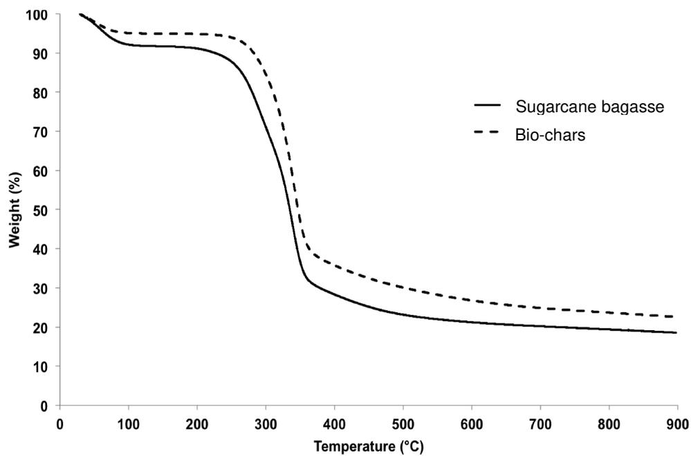
Figure 3. ATG curves of the sugarcane bagasse and bio-chars
