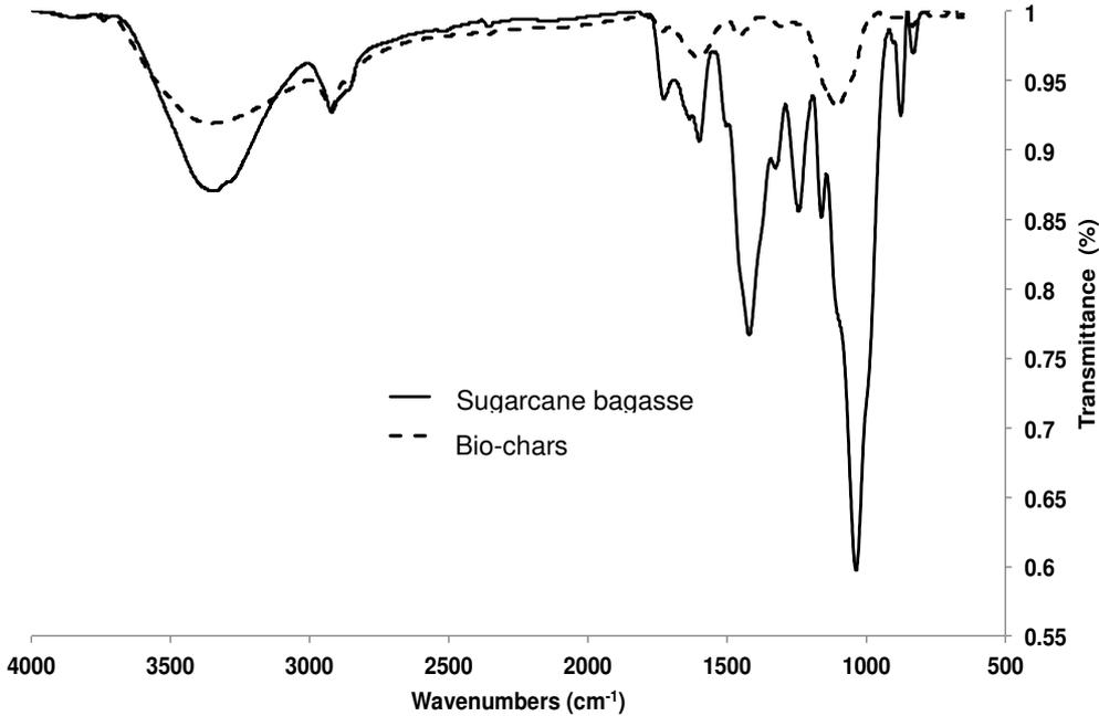
Figure 2. FTIR spectra of the sugarcane bagasse and bio-chars
