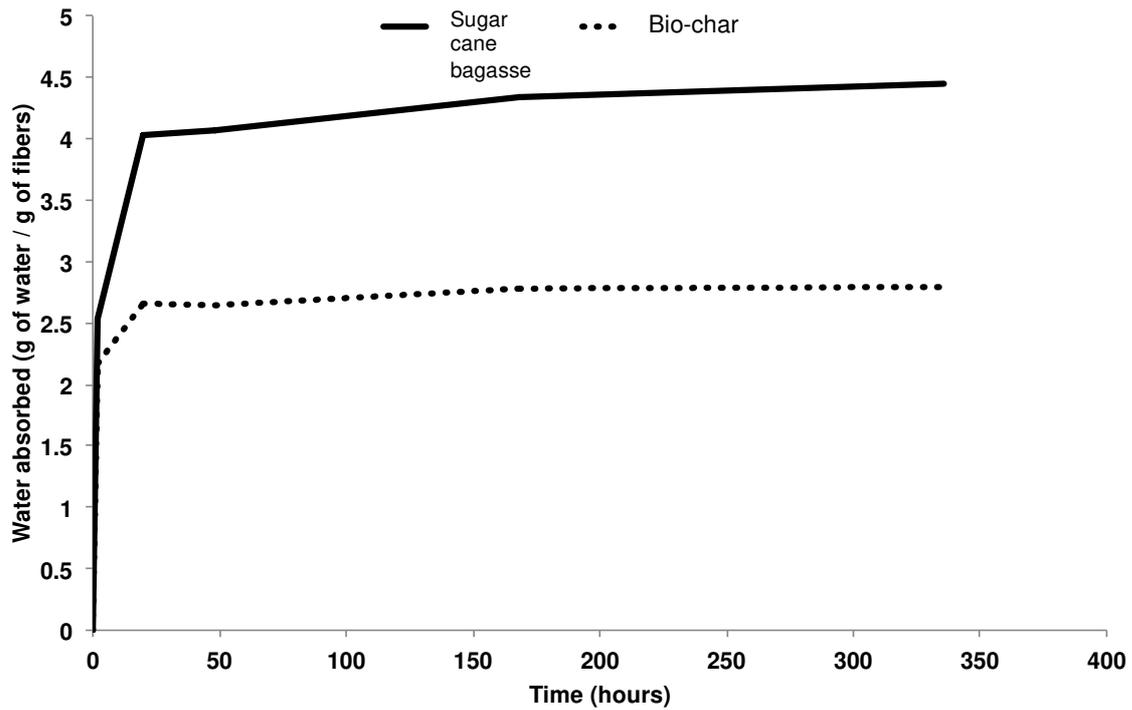
Figure 5. Evolution of water absorbed by the sugarcane bagasse and bio-chars with time
