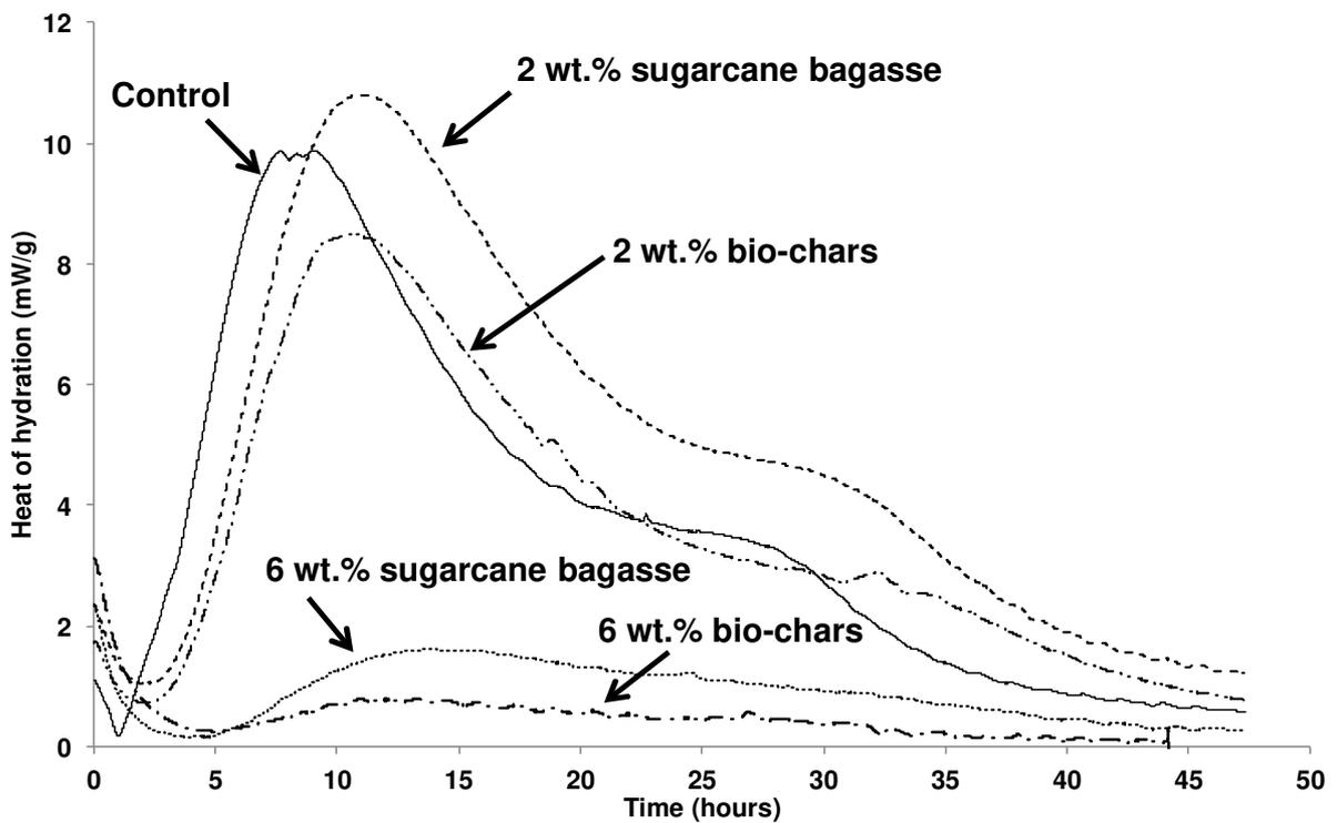
Figure 6. Heat of hydration of cement pastes containing 0, 2 and 6% by weight of bio-chars or sugarcane bagasse
