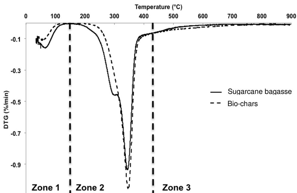
Figure 4. DTG curves of the sugarcane bagasse and bio-chars
