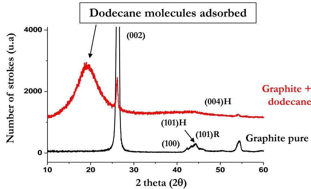
The position of the diffraction peaks corresponding to the interfering spaces are not modified in the presence of the organic liquid.
