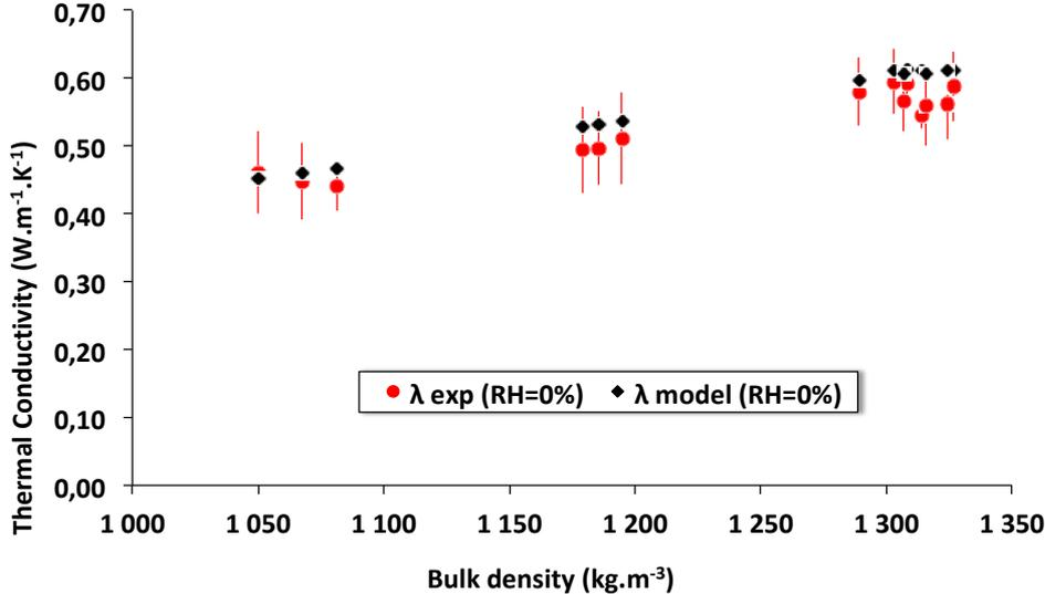
Figure 9: Thermal conductivity varying with bulk density: comparison between theoretical calculations and experimental results (RH=56%)
