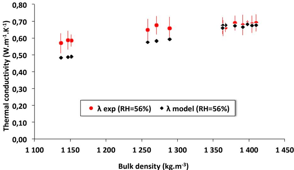
Figure 10: Thermal conductivity varying with bulk density: comparison between theoretical calculations and experimental results (RH=100%)
