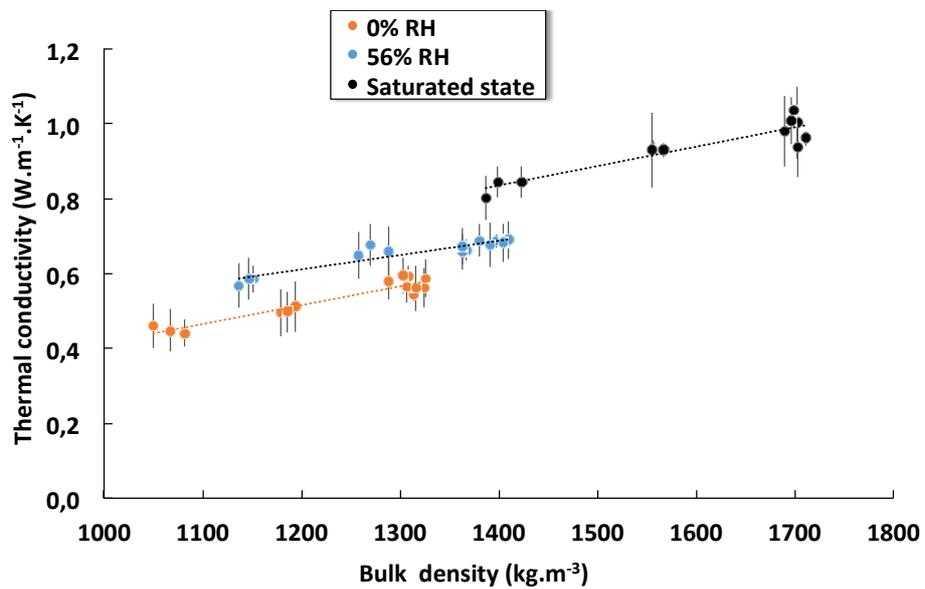
Figure 8: Comparison between theoretical calculations and experimental results of thermal conductivity of dry composites according to bulk density
